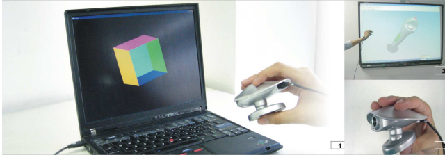
Figure 1. Picture 1 shows the platform of experiment. Picture 2 uses UCam to view a 3D object in large display. Picture 3 shows the handheld camera used in UCam.
