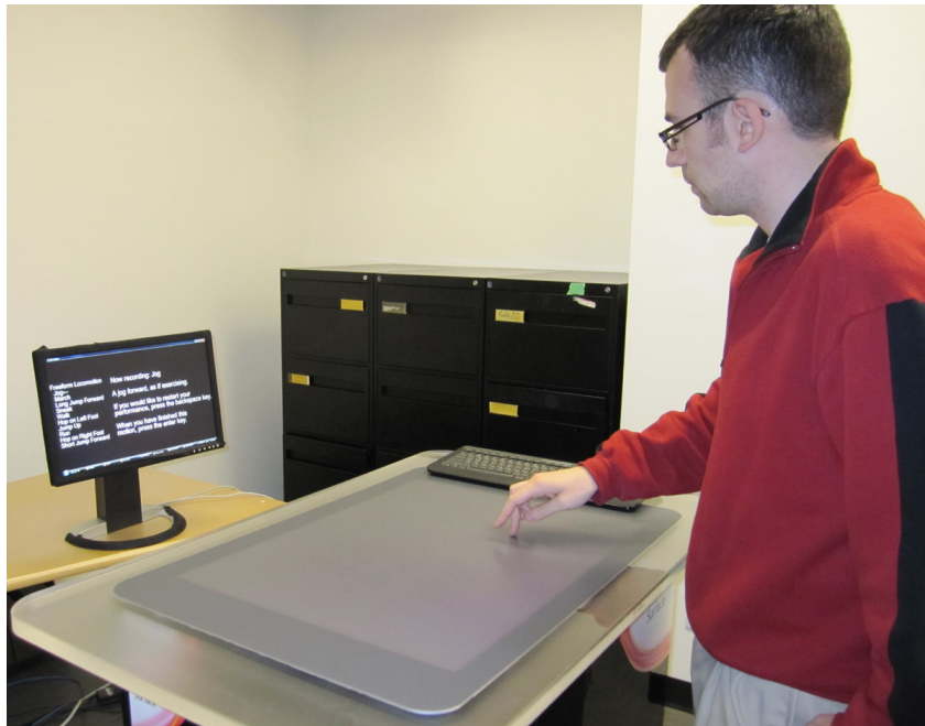
Figure 4.2: Equipment used to study hand performances. Directed by instructions on the external monitor, participants were free to move around the Microsoft Surface, which captured contact data, while their above-surface motions were video recorded.
