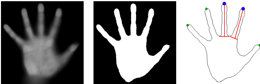
Figure 4.8: While the Surface can provide approximate depth images (left), appropriate thresholding yields a hand shape (middle) which can be automatically analyzed to identify and measure fingers (right).
