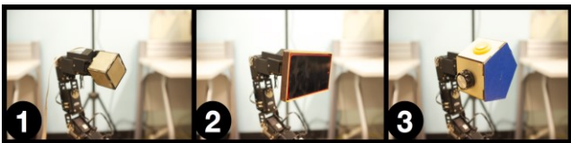
Figure 7: Examples of endpoints used for input. (1) Force sensors detect grasping, (2) a phone used for its capacitive touch sensor (3) physical UI controls enable fine-grained input and physical feedback.
