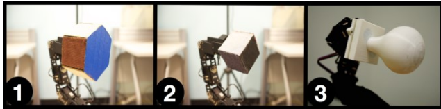
Figure 6: Endpoints synthesize physical features: (1) various materials of a shoe (2) several textures for a clothing scenario (3) a snake head used to ‘attack’ the user.
