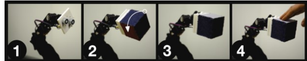
Figure 3: Surfaces are synthesized by (1) the robotic arm; (2) with an attached endpoint. By rotating the endpoint to present the desired texture (3), the surface texture presented to the user (4) aligns to the virtual object.
