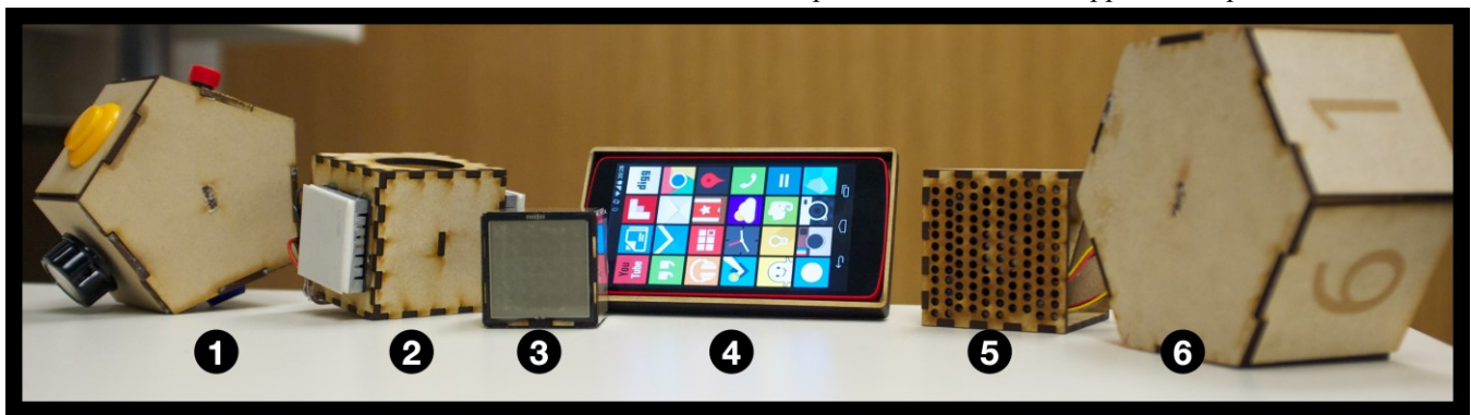
Figure 2: Examples of different endpoints that can be attached to simulate surface characteristics. (1) Physical controls, (2) Peltier Pad for heating/cooling, (3) whole object interaction via pressure sensing, (4) touchscreen, (5) air flow, (6) six sided texture base.
