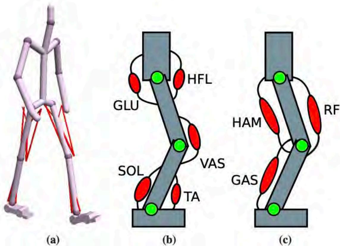
**Figure 1:** *Humanoid model. (a) Sixteen Hill-type MTUs, shown in red, generate torques for the hips, knees, and ankles. Note that the back joint is not rendered for aesthetic reasons. (b) Five uniaxial muscles in each leg produce flexion or extension torques at single joints. (c) Three biarticular muscles in each leg generate torques at pairs of joints. See Section 3 for details.*
