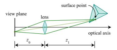
More generally, for the thin lens model, if  $z_1$  is the distance from the center of the lens (i.e., the nodal point) to a surface point on an object, then for a focal length |f|, the rays from that surface point will be in focus at a distance  $z_0$  behind the lens center, where  $z_1$  and  $z_0$  satisfy the thin lens equation:
