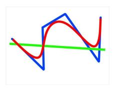
Figure 15: The line (green) will always intersect the curve less often than or as many times as the control polygon.
