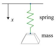
A spring has resting length l and stiffness k. Deformation force is linear in the difference from the resting length. Hence, a spring's internal force, according to Hooke's Law, is  $f^s(t) = k(l - x(t))$ .
