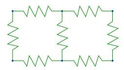
Let the *i*th mass,  $m_i$ , be at location  $\bar{p}_i(t)$ , with elements  $x_i(t)$ ,  $y_i(t)$ ,  $z_i(t)$ . Let  $l_{ij}$  denote the resting length and  $k_{ij}$  the stiffness of the spring between masses i and j.
