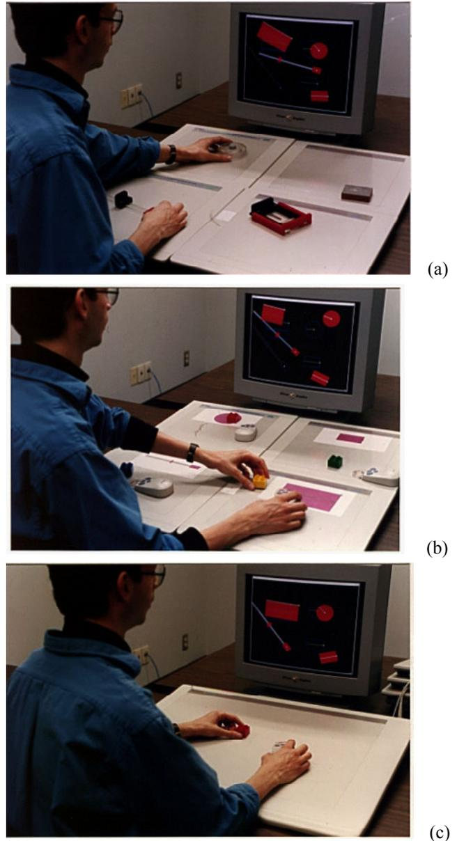
**Figure 5.** Experimental set-up: (a) space-multiplex with 4 specialized devices using 4 tablets, (b) space-multiplex with 4 puck and brick pairs of generic devices using 4 tablets and (c) time-multiplex with one puck and brick device operating on a large tablet.
