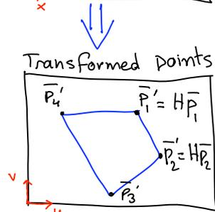
Linear warps correspond to every possible distortion of a square created by moving its vertices to arbitrary locations
