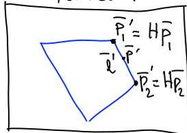
So the transformed points satisfy a line equation too, with line coordinates  $\bar{l}^T H^{-1}$
