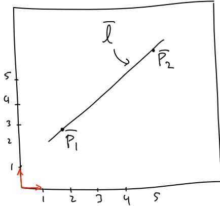
Calculating the parameters of a line through two points with homogeneous coordinates  $\bar{P}_1, \bar{P}_2$
