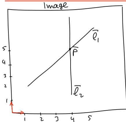
Calculating the homogeneous coordinates of the intersection of two lines  $\bar{l}_1, \bar{l}_2$
