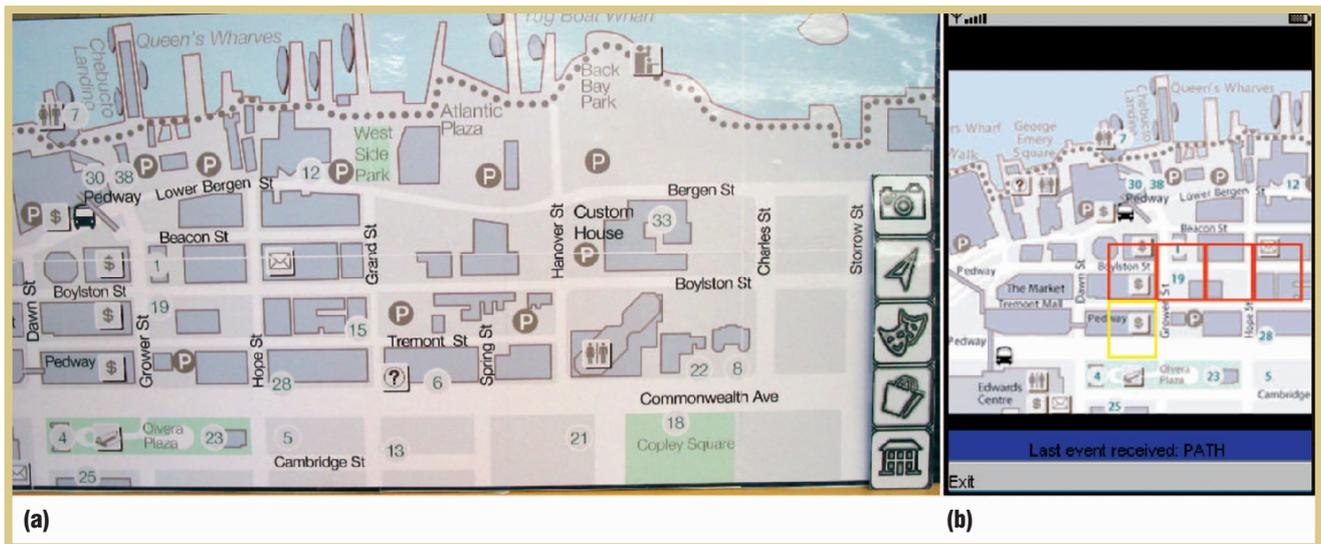
Figure 4. The second Marked-Up Maps prototype: (a) A paper map used with the prototype. (b) One way the prototype provided feedback was to highlight selected map grid squares in red.
