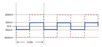
Figure 6. The square wave signal in Component Recognition. The period of the square wave is 0.02 seconds and the amplitude is initially set to 500mV (Blue) which can be adaptively increased to the maximum voltage, 2000mV (Red).
