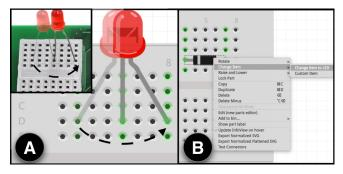
Figure 11. (A) As one lead of a component is detached and then inserting to the another hole on the breadboard, CircuitSense will automatically modify the pin location on the virtual breadboard. (B) For the component unable to be distinguished such like an LED and diode, users can revise the type of component by our custom software extension.
