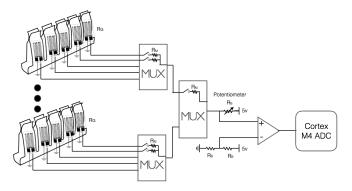
Figure 4. The circuit design of Pin Location Sensing. All sensing clips are connected to two-stage cascade of multiplexers. For measuring the small change in resistance of the strain gauges, the resistance( $R_B$ ) of balanced resistor is equal to the sum of two inner resistance of multiplexers( $R_M$ ) and the basic resistance of strain gauge( $R_G$ ). ( $R_B = 2 \times R_M + R_G$ ). The potentiometer is used for minute adjustment in resistance.
