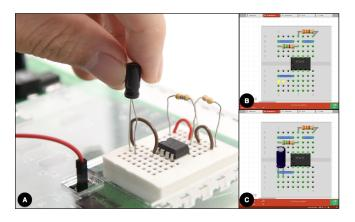
Figure 1. CircuitSense is a hardware+software system that facilitates automatic virtualization of physical circuit designs. (A) When developers place wires or electronic components on our CircuitSense breadboard, (B) Pin Location Sensing determines the location (highlighted in yellow) and the number of pins, followed by (C) Component Recognition identifying the type of that electronic component, and CircuitSense generates the corresponding software representation ultimately.
