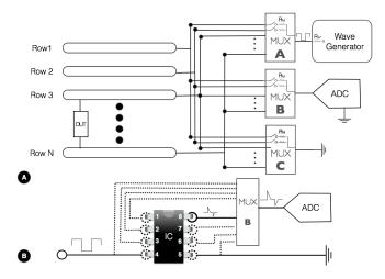
Figure 7. Hardware design for Component Recognition System (A) Each Row of Breadboard is connected to 3 multiplexers respectively for squared-wave input, data collection device and ground. (B) Multiplexer B switches between 8 pins of IC to retrieve waves passed to ADC.
