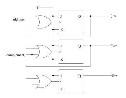
3. What is the output sequence of the following "counter", after it gets established in its cycle?
