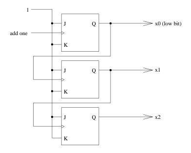
Draw a three-bit counter with *two* inputs: an "add one" input such as above, and a "complement" input which toggles all three bits (e.g. 010 will become 101).
