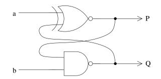
(a) List all of the possible stable states for each of the possible four input combinations, by stating the outputs of each gate (i.e. values P and Q).
