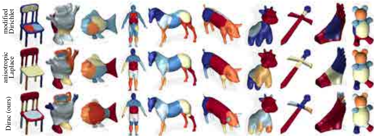
Figure 11: Segmentation results using identical parameters for a variety of operators. In addition to finding strong feature curves, our extrinsic operator tends to resolve small features like ears and toes, and avoids spurious “triple points” or arbitrary patch boundaries that convey no clear geometric information (beyond an equipartition of area).
