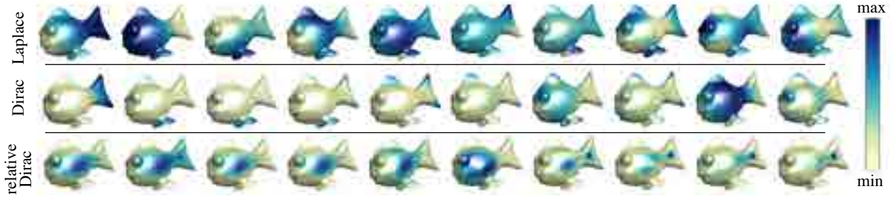
Figure 6: Eigenfunctions of several operators. Both the Dirac and relative Dirac operators put more emphasis on extrinsic curvature, with the relative Dirac operator placing special emphasis on flat regions.
