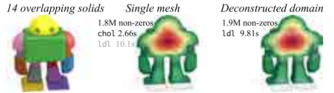
Figure 17: Traditional mesh-union then tetrahedralization succeeds on this example, enabling an ad hoc performance comparison. System matrices for solving the Poisson equation require similar memory; however, our MATLAB implementation uses LDLT on our resulting Lagrangian: about 3.7\times slower than Cholesky, here.
