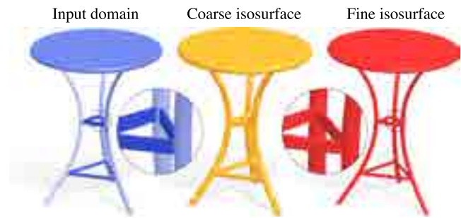
Figure 4: This seemingly innocuous union (left) causes the conforming Delaunay method TETGEN [Si03] to fail. Implicit or query-based methods have trouble capturing fine structures (middle) without resorting to high resolutions (right).
