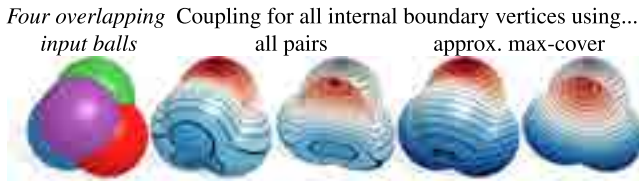
Figure 12: Boundary coupling across all sub-domain pairs leads to messy locking near the overlap boundary (6001 constraints). Instead, our heuristic keeps exactly one constraint per overlap boundary vertex (3893 constraints).
