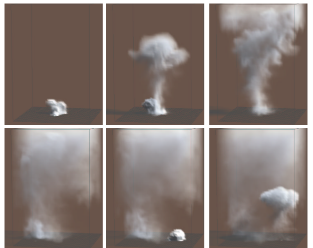
Figure 7: Six frames rendered using our interactive hardware renderer of the smoke. The simulation time for a 40 \times 40 \times 40 grid was roughly 1 second/frame.
