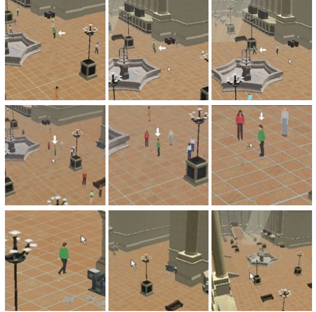
Figure 6: Row 1: A fixate sequence. Row 2: A zoom sequence. Row 3: Camera returns to its default settings upon losing the pedestrian; it is now ready for another task.
