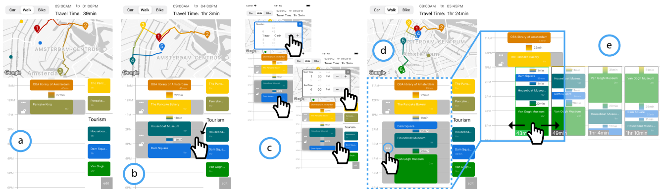
Figure 5: Before (a) and after (b) adding an as-many-of group to the schedule. The group automatically schedules the largest subset of locations that can fit within the block’s duration, in the arrangement that results in the least possible travel time. The pre-existing one-of group also updates to minimize travel time upon this change (a to b). The overall block duration of a group can be adjusted, as can the durations of independent destinations within an as-many-of group (c). The map updates according to such changes (d). Alternative schedule permutations can be browsed in-situ by tapping on the “...” icon (e).
