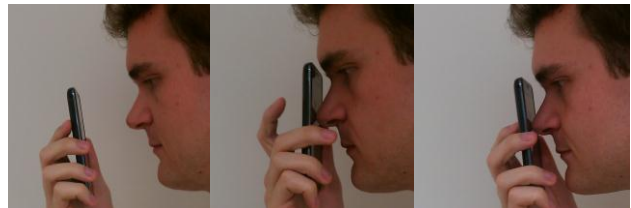
Figure 5. The touch + tap gesture activates manipulation mode. The user touches the object to be manipulated with their nose input and taps on the back of the device.
