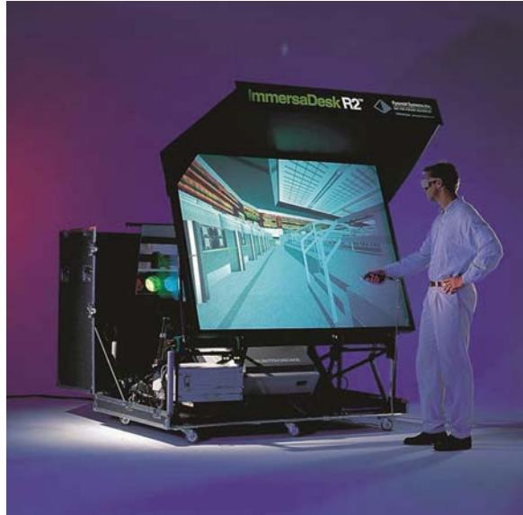
Fig. 12.2 The ImmersaDesk [14] utilized a stereoscopic display, enabled with shutter glasses (ImmersaDesk™ photo courtesy of the Electronic Visualization Laboratory at the University of Illinois at Chicago. ImmersaDesk is a trademark of the University of Illinois' Board of Trustees)
