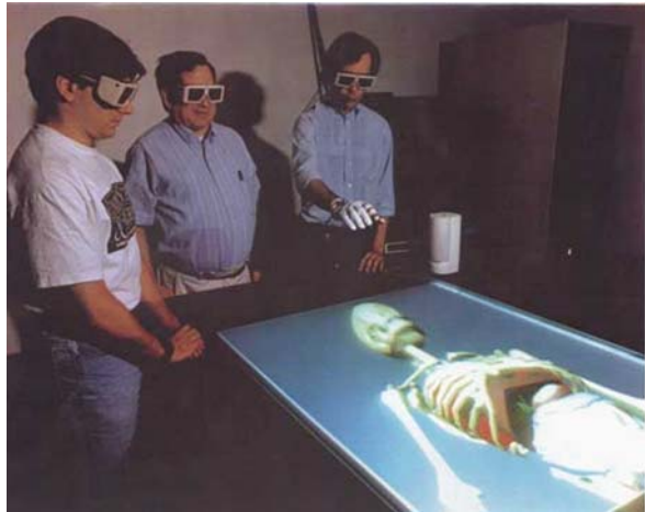
Fig. 12.6 The responsive workbench's display was constrained to the table, with false 3D created through shutter glasses
