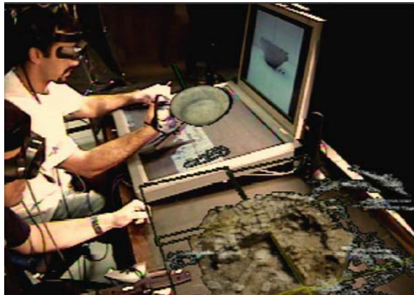
Fig. 12.8 Benko et al.'s hybrid virtual environments used a head-mounted display to insert imagery into the space between the user and the table
