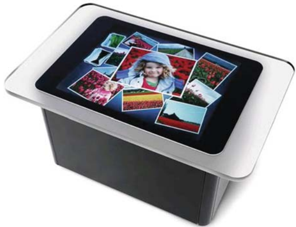
Fig. 12.1 The microsoft surface table. A multi-touch input device with a two-dimensional display
