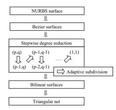
Fig. 3. Overall procedure of parametric-surface tessellation.
