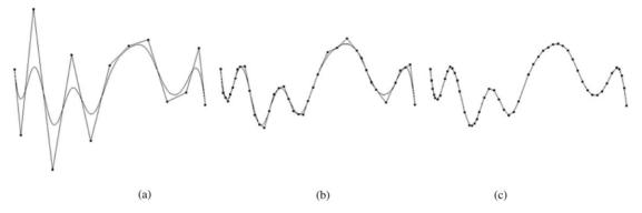
Fig. 2. Parametric-curve polygonization method based on stepwise degree reduction: (a) given cubic B-spline curve, (b) quadratic Bezier curves, and (c) resulting piecewise-linear approximant.
