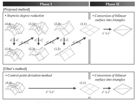
Fig. 4. Two-phase approximation approach.
