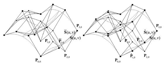
Fig. 6. u-directional stepwise degree reduction of Bezier surface of degrees (3, 3).
