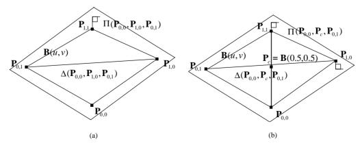
Fig. 11. Conversion of bilinear surface into triangles.
