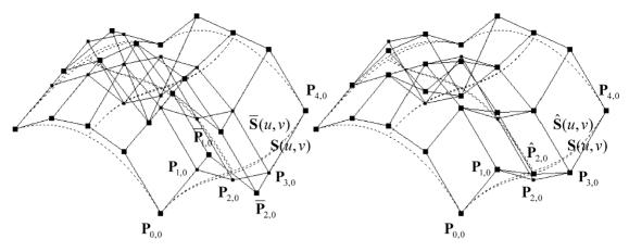
Fig. 5. u-directional stepwise degree reduction of Bezier surface of degrees (4, 4).
