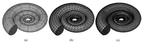
Fig. 12. Parametric-surface tessellation of nautilus-shell shaped surface: (a) bicubic B-spline surface, resulting piecewise-planar approximants with pre-defined tolerance, (b) 2.0, and (c) 1.0.
