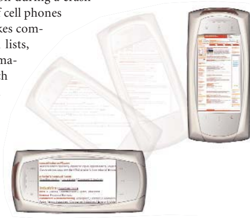
A motion-sensing phone changes display orientation.
