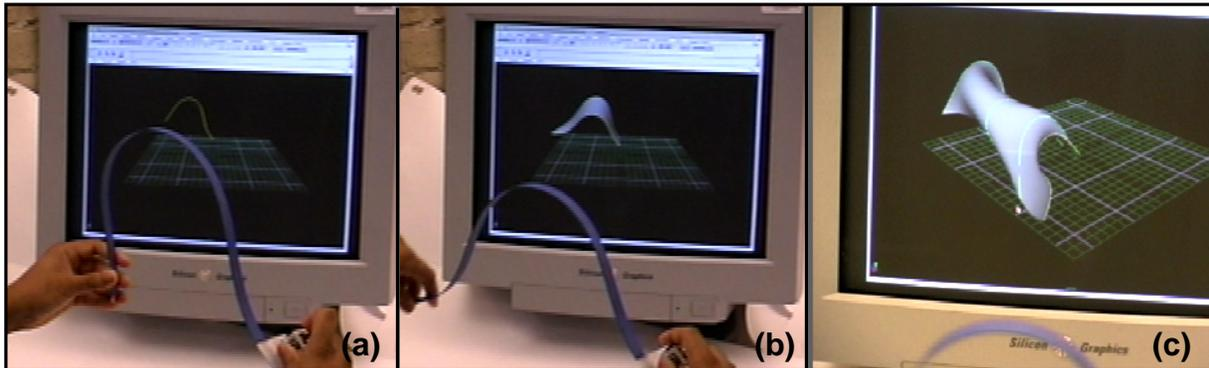
*Lofting a surface with ShapeTape. (a) Placement of initial profile curve. (b) Dragging out first section of the lofted surface. (c) The final surface lofted over five interactively placed profile curves.*
