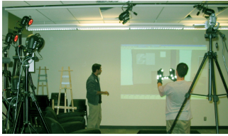
Figure 1: The DirectCam system in use. Hand motion is tracked using reflective markers on gloves and a Vicon optical motion tracking system. This provides the interface to scene editing appropriate for a large display of the scene.
