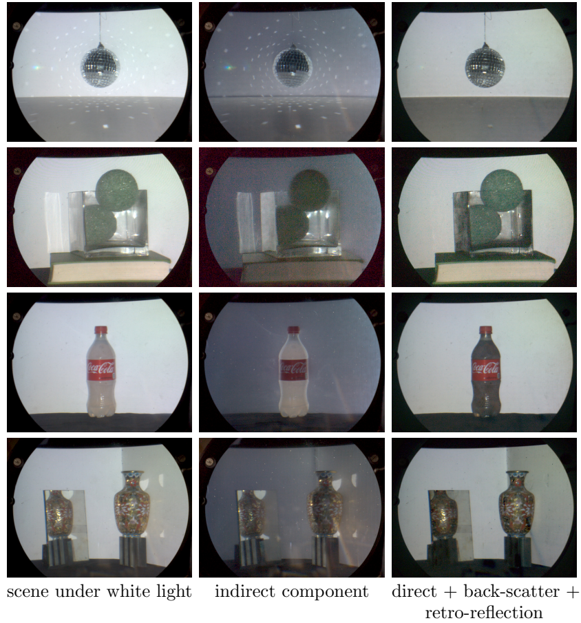
Figure 3.9: Left to right: Photo of scene under white light, indirect component of scene captured by a single RAW photo, direct component computed by subtracting the indirect image from the scene under white light. No processing was done on the photos, other than a resize, flip, white balance, gamma correction and crop. All scenes use 512 mask and illumination codes, with the exception of Row 4 which uses 1024 codes. Row 1: A disco ball produces specular indirect transport across the scene, with diffuse inter-reflections occurring near the edge of the floor. Optical probing cleanly separates the photo into its direct component and its indirect component, which contains inter-reflections and specularities. Row 2: A scene composed of two styrofoam balls inside a glass container generates specular reflections, sub-surface scattering and caustics. We used small aperture to photograph this scene in order to avoid pixel saturation due to caustics. The photo is slightly noisier as a result. Row 3: A coke bottle filled with milky water strongly scatters light that enters the bottle. Row 4: Observe that the direct component contains none of the light that is reflected by the mirror (left) onto the vase (right) and the wall. However, the mirror does not appear black in the direct photo even though it has little to no direct component. This is because of back-scattering and retro-reflection (Figure 3.2(c)): light leaves a projector pixel, hits the mirror at a point, diffusely reflects off the wall, then hits the mirror at the same point, and returns to the same pixel. This light path will always contribute to the diagonal of the transport matrix and cannot be distinguished from direct illumination using methods that rely purely on intensity, and without regard to arrival time. Note that according to Eq. (3.9), the variance of stochastic diagonal estimation may be higher for indirect specular transport than for diffuse transport. To compensate for this, we used 1024 codes for this scene.
