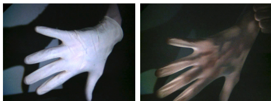
Figure 4.16: Frames from a conventional video (left) and RAW non-epipolar video (right) of a tight-fitting latex glove. Note the seemingly transparent nature of the glove in non-epipolar mode. The hand is dark in regions where the glove makes contact with the skin; otherwise, light scatters within cavities between the glove and skin.
