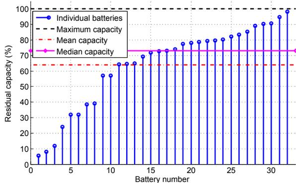
Figure 2: Residual capacity of a sample of discarded laptop battery packs
