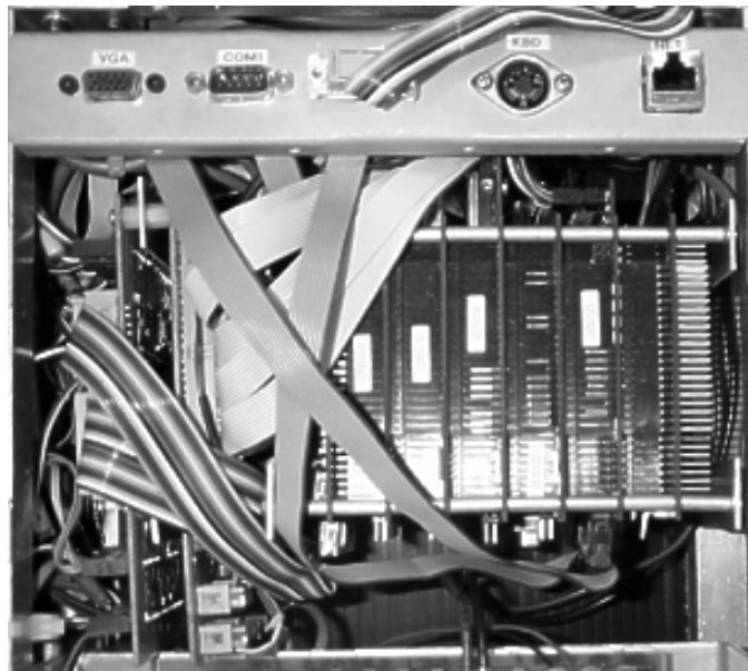
Figure 3.6: PC104 computer mounted inside robot chassis. Designed custom I/O boards can be seen on left hand side of image.
