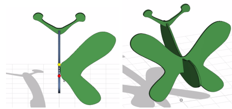
Figure 6. A planar section contour drawn principally on one side of the slit (left), is mirrored across slit and smoothly joined (right).
