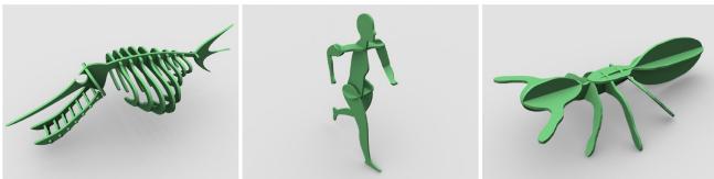
Figure 3. Planar sections can represent non-manifold scaffolds (left), conform partly (middle), or entirely (right) to 3D object contours.
