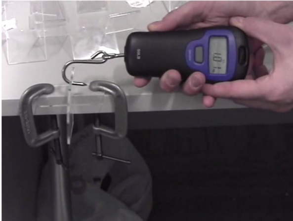
Figure 5.24: (Left) Our physical experiment where force was applied to planar section joints along three major axes to determine the amount required for fracture. (Right) Fractures occur in a consistent pattern, across planar sections.
