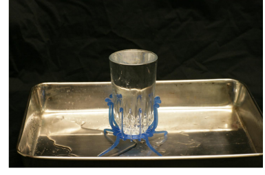
Figure 5.26: Four variations of an object intended to hold a glass of water. (First row) The first variation has three thin legs, which fracture before a glass can be filled. (Second row) A variation with 4 thin legs, which also fracture under the weight of a glass of water. (Third row) A stronger variation with three thicker legs is able to withstand the weight of a full glass of water, but our system warns of a potential fracture where the legs and central disc meet. (Fourth row) An even stronger 4 leg design also handles the weight of a glass of water, and our system reduces the warning of potential fracture where legs and central disc meet.
