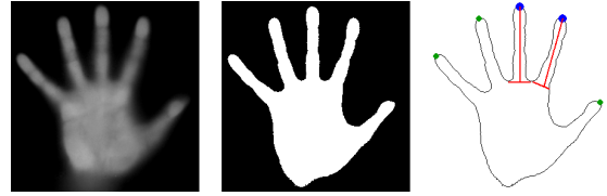
Figure 8: While the Surface can provide approximate depth images (left), appropriate thresholding yields a hand shape (middle) which can be automatically analyzed to identify and measure fingers (right).
