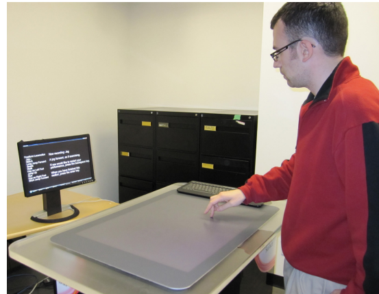
Figure 2: Equipment used to study hand performances. Directed by instructions on the external monitor, participants were free to move around the Microsoft Surface, which captured contact data, while their above-surface motions were video recorded.
