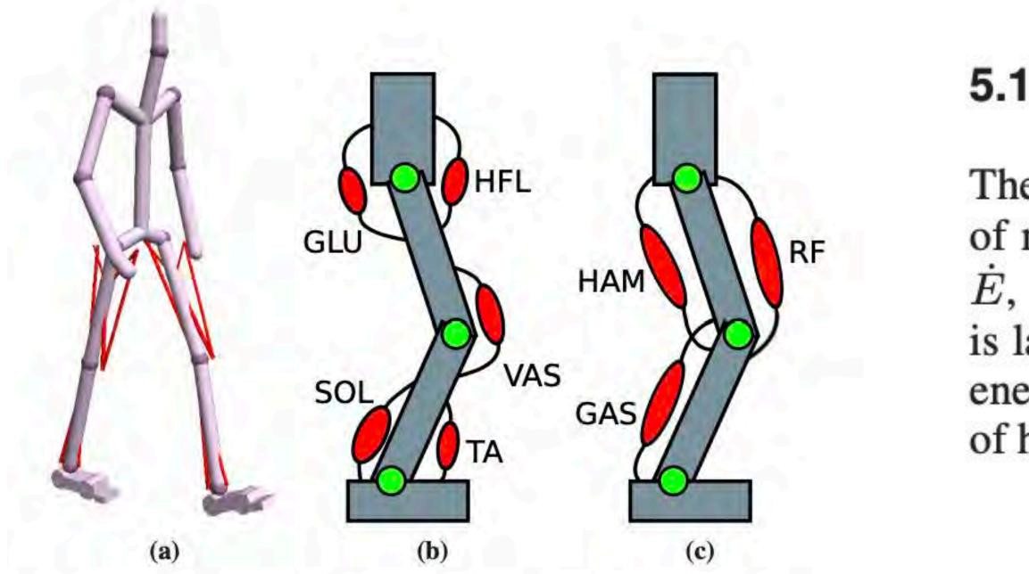
Figure 1: Humanoid model. (a) Sixteen Hill-type MTUs, shown in red, generate torques for the hips, knees, and ankles. Note that the back joint is not rendered for aesthetic reasons. (b) Five uniarticular muscles in each leg produce flexion or extension torques at single joints. (c) Three biarticular muscles in each leg generate torques at pairs of joints. See Section 3 for details.
