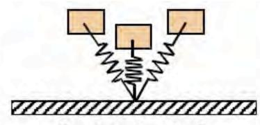
Spring-loaded inverted pendulum (SLIP)
