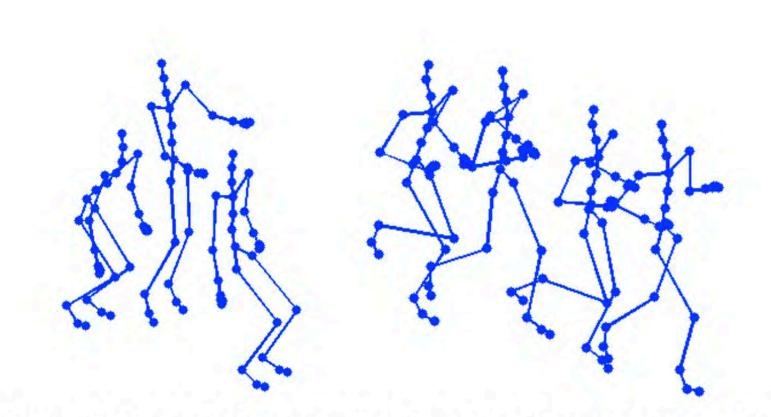
Figure 11. **Tracking human motion.** Reconstructions of a jumping and a jogging sequence with an image noise of variance 4.
