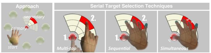
Figure 4. Study interface: 8 approach directions (N, NE, E, SE, S, SW, W, NW) from the start button to the primary target, and three different serial target selection techniques: *Multi-tap*, Sequential, and Simultaneous.
