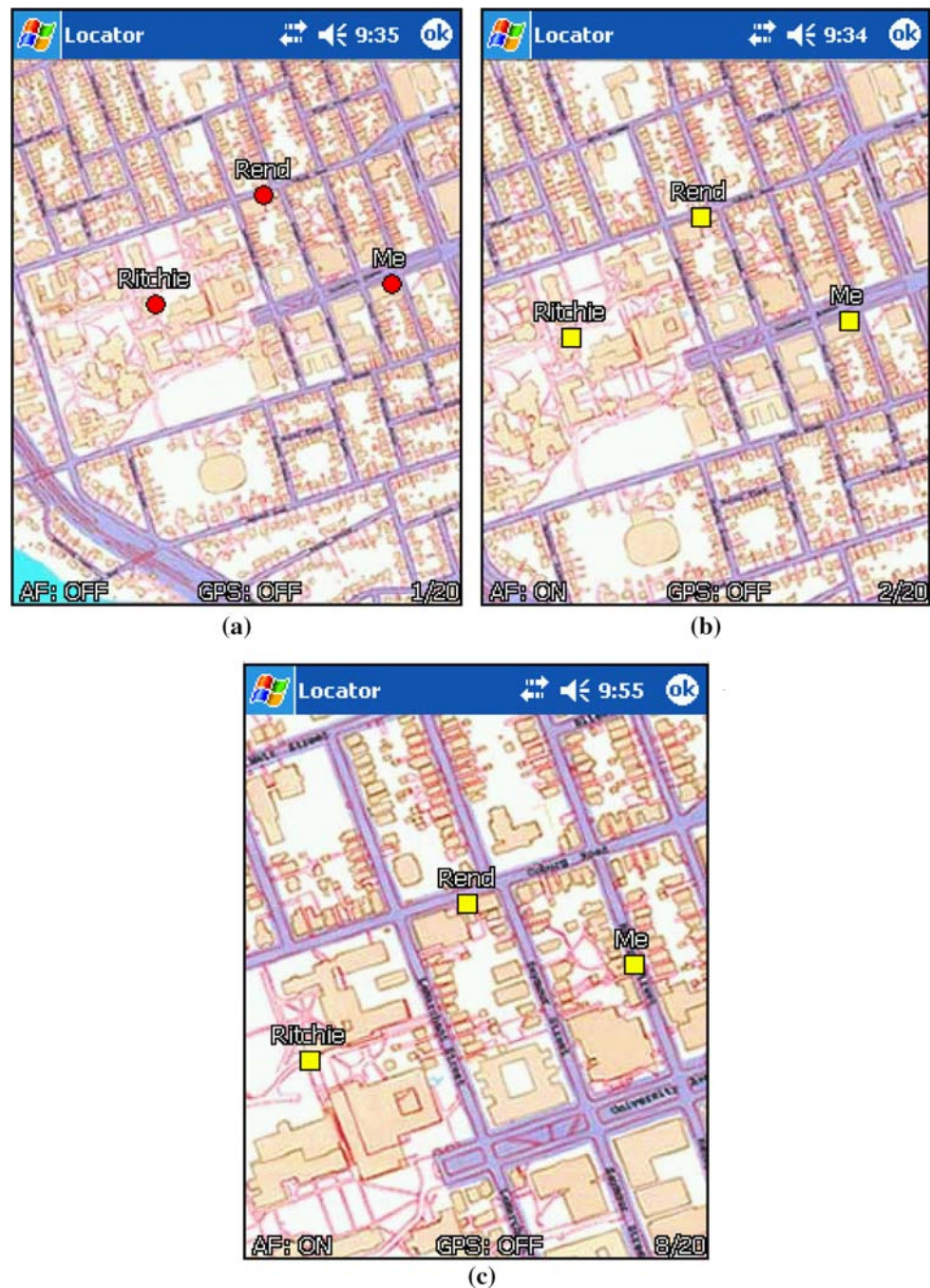
Fig. 2 The location-aware map application used in study 2 (autofocus). In a the participant ('Me'), their partner ('Ritchie') and the rendezvous ('Rend') are initially not selected as focus locations. The participant selects all three locations ( b ) as focus locations. As the proximity between the 3 locations change ( c ), autofocus zooms and pans the map appropriately
