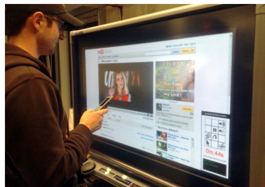
Figure 1. A user controlling the playback of a YouTube video on a public display from his mobile phone using BlueTone.
