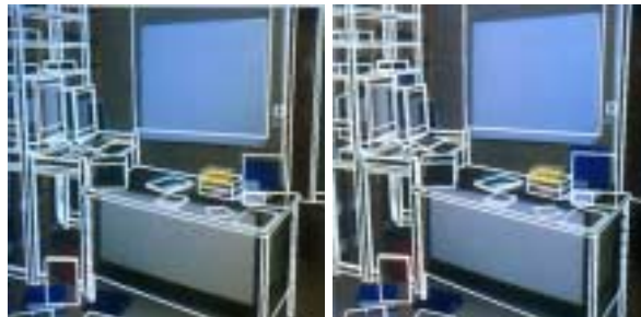
FIG. 2.6. Recognition results using the reconstructed facets of figure 2.4. The original stereo pair is visible on the background and the white wireframe shows the position of the part of the database that the algorithm found.
