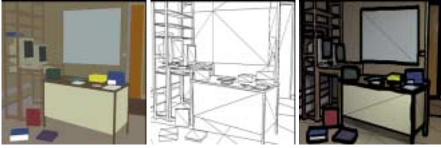
FIG. 4.7. Left image: index buffers with a specific color by group. Middle image: hidden-surface image. Right image: combination of the the left and middle image, adding an edge detector to remove positioning problems of the 3D model.
