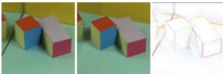
FIG. 4.11. The original image is on the left. The middle one is the result of the \rho convergence after only 3 re-rendering iterations with specular processing. The right image is the difference between the real and the synthetic image, where the darkest areas correspond to the biggest errors.
